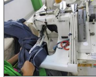
External photo(s) of the production unit(s) NC Image 7.17-Feed of the arm sewing machines in the sewing section did not have needle guards...JPG
