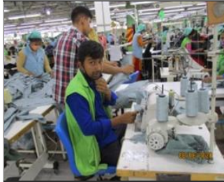
External photo(s) of the production unit(s) NC Image 7.6-Overlock sewing machine operators in the sewing section were not using mask.JPG
