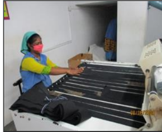
External photo(s) of the production unit(s) NC Image-7.6-Fusing machine operators in the fusing room were not using hand gloves...JPG
